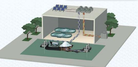
Ice shavings from the Zamboni are dumped into a shallow pit and used to additionally cool water from a geothermal well. This cool water is then pumped through the DH units, providing the necessary heat extraction. Meanwhile, free heat from solar thermal panels and the microturbine exhaust create hot water that provides the heat necessary for regeneration.
